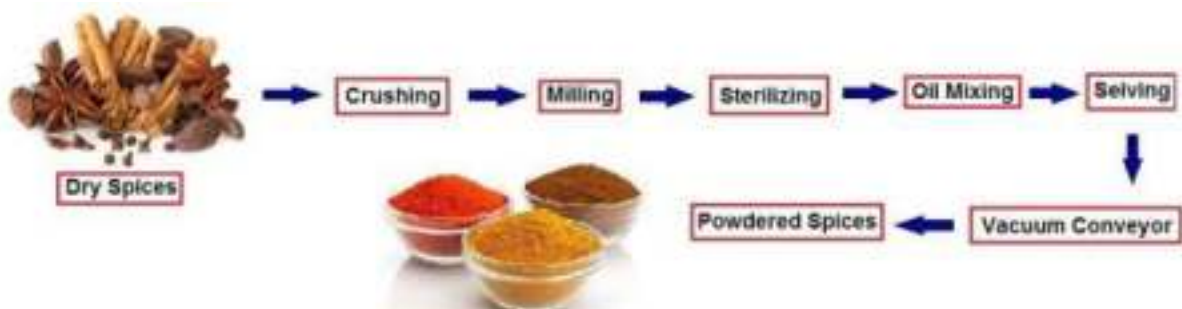
Fig 3.2.2 Flowchart for whole spices manufacturing
