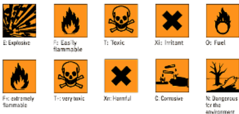
Fig. 5.13.2: Chemical hazard safety signs
