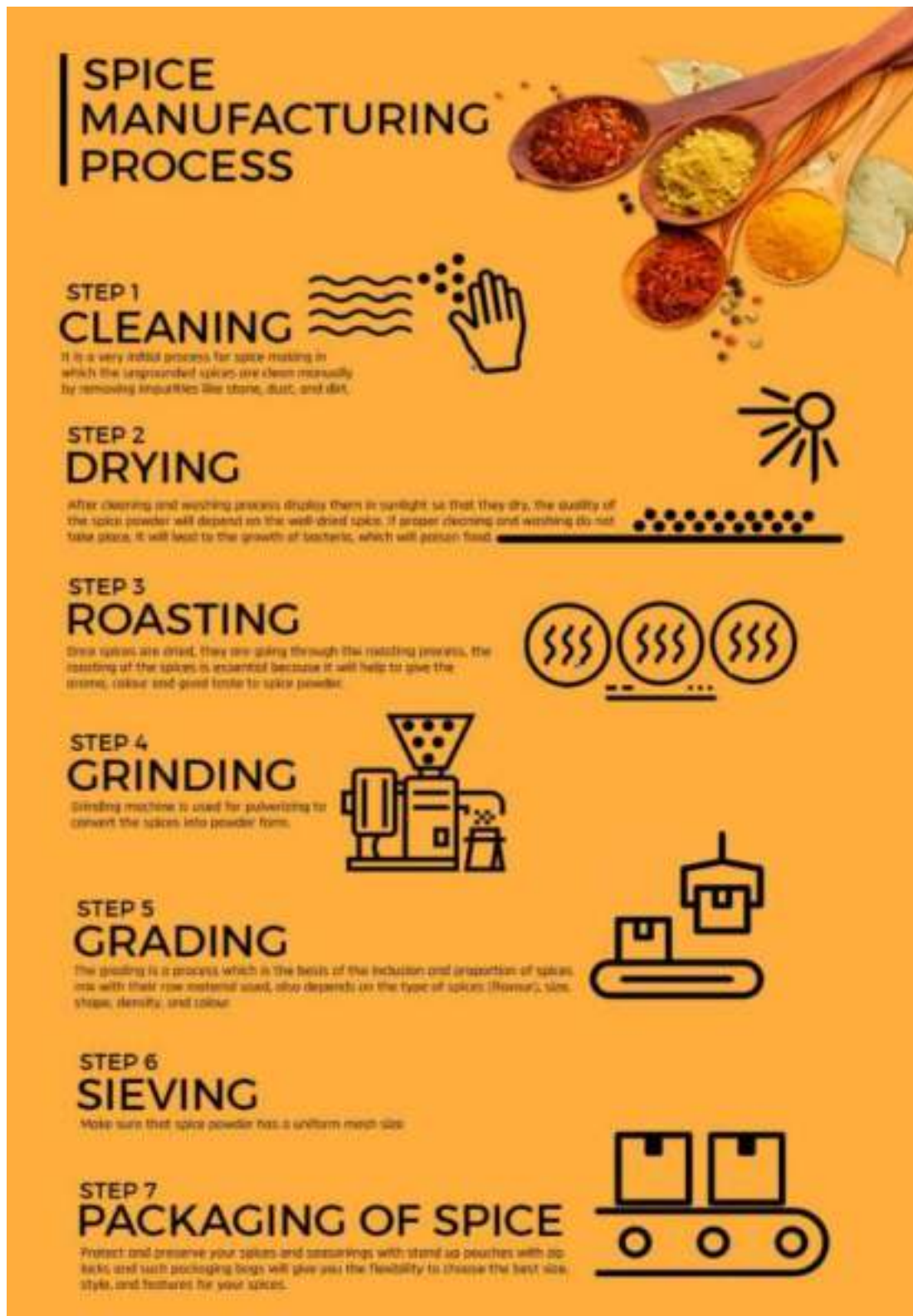
Fig 2.1.5 Product flow chart of powdered spices manufacturing
