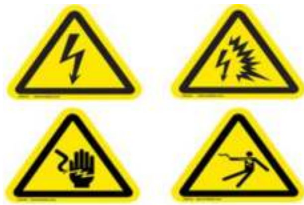
Fig. 5.3.2: Electrical hazard symbols
