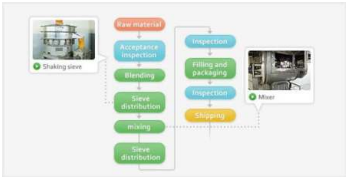
Fig 3.2.7: Seasoning Manufacturing Process
